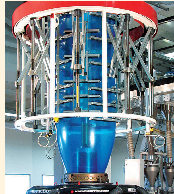
The VARIOCAGE film calibration unit ensures tight tolerances.
