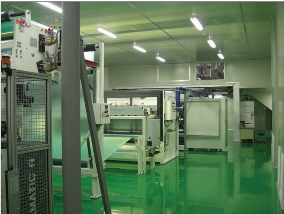
FILMEX cast film line for the production of surface protection films under clean room conditions
