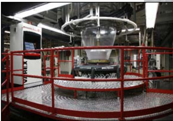
One of Ampac Flexibles' 3-layer VAREX extrusion lines
